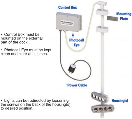
the screws on the back of the housing(s) to desired position.
