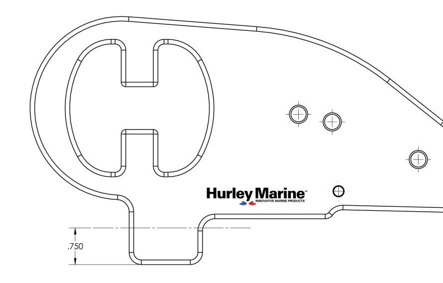
NOTE: When swapping H2O 6", 8" or 10" davit to H2O 36" davit the customer will need to cut off .75" of the H2O cradle's foot. This is measured from the bottom of the H2O foot as in the image above. This is due to the added height of the H2O 36" mount which sits between the H2O cradle and button mount plates.
