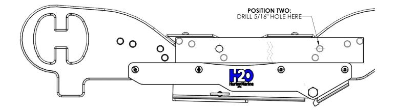
Note: New style cradles will have two dimples on the side where holes should be drilled.
