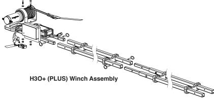
Inspection and tightening of screws, nuts and bolts should be performed weekly. Always clean the davit system with fresh water when it is used in a corrosive environment.
