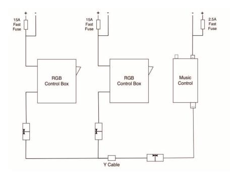
The RGB control cable from the music controller can be extended up to 100 feet using CAT-5 network cable or 4 conductor telephone cable.
