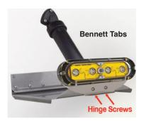
Remove the 1/4"-20 x 3/4" Philips head machine screws from lower hinge. Place Trim Tab Brackets on and reinstall screws. Different hole patterns for other leveling systems.
